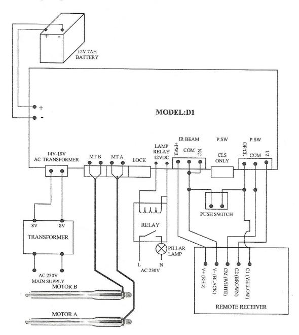
NOTE: USE 8V & 8V FOR TRANSFORMER VOLTAGE
